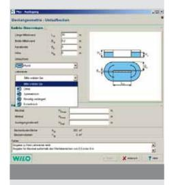
Using our Mixer Select configuration software, the right mixers for any tank shape and size can be determined quickly and easily.
