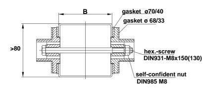
The fixing can be realized onesided (EBA 1) or two-sided (EBA 2) on the stainless steel diffuser pipe (rectangular or round) by using the ENVICON adapters (diameter of the hole 40 mm).
