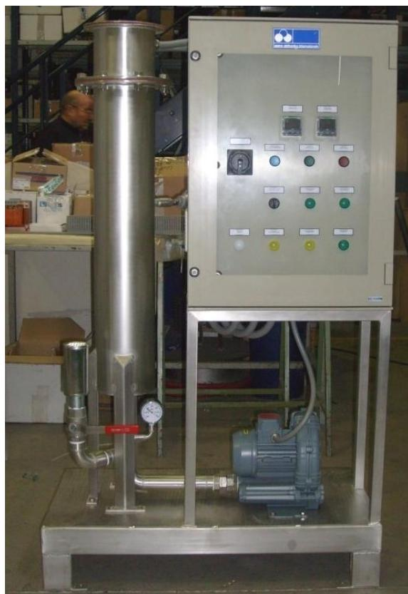
*The gas leaving the ozone contact system will be freed from any possible remaining traces of ozone in the vent ozone destruction plant. The destruction of ozone is based upon the principle of thermocatalytic decomposition.*
