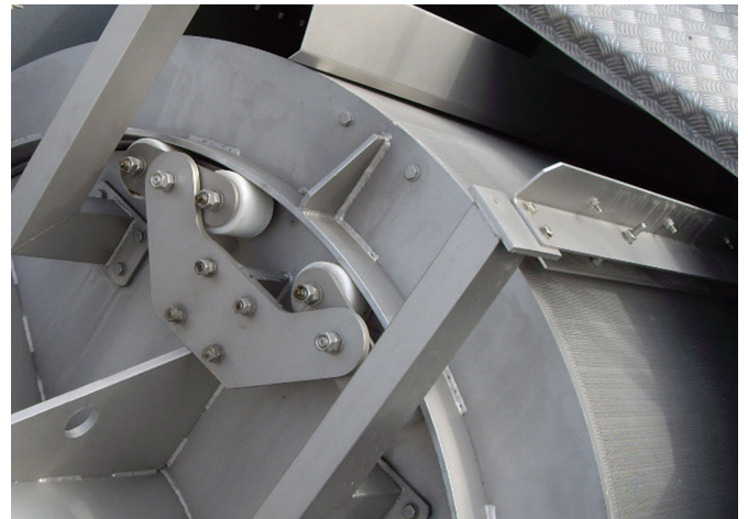
Stable roll bearings in the Meva MDS
