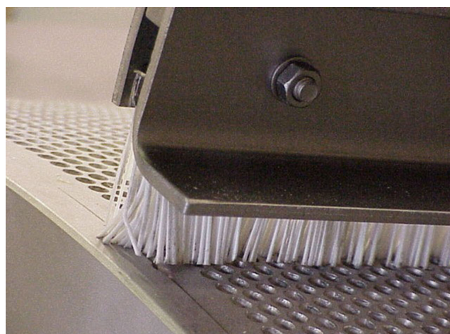
Easily replaced nylon brush
