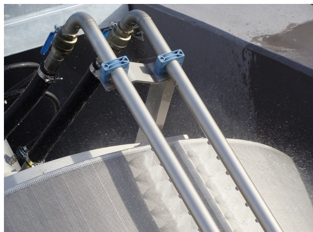
Overlapping flushing system of the Meva MDS
